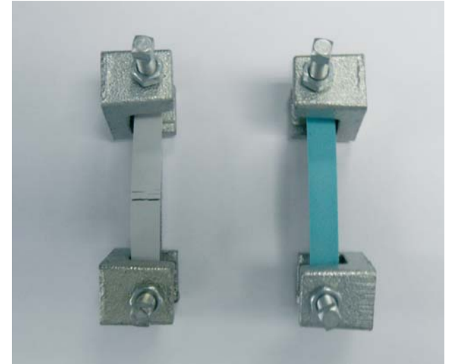
Clamped Charpy bars after immersion in olive oil, left: PC/ABS FR right: PC/PBT FR (EXP 1950)
