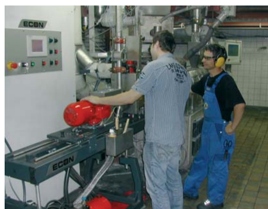
Underwater granulation in progress
